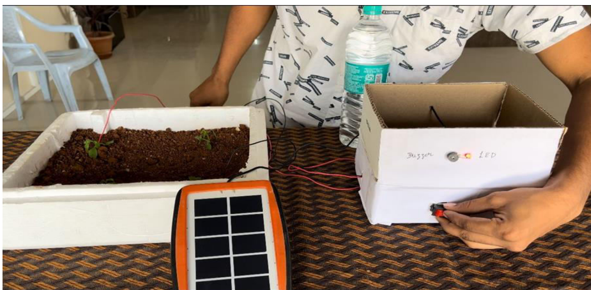
Placing the Resistors in the Dry soil the LED Bulb and the Sound Buzzer Gets ON
